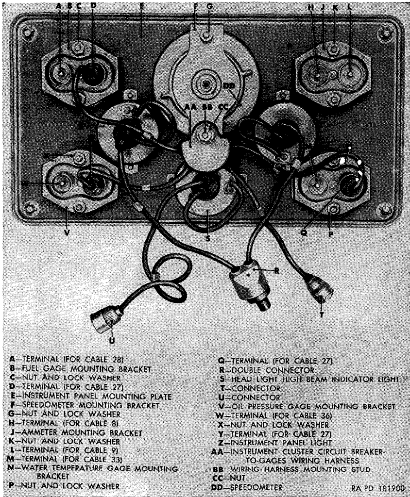
Figure 114. Instrument cluster (M38A1)—rear view.
