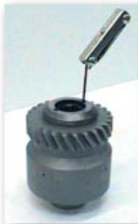
Step P2 Using a 7/64" Allen wrench, remove the socket head screws holding the beveled spacer. (Early model Warn units used 2 roll pins).
