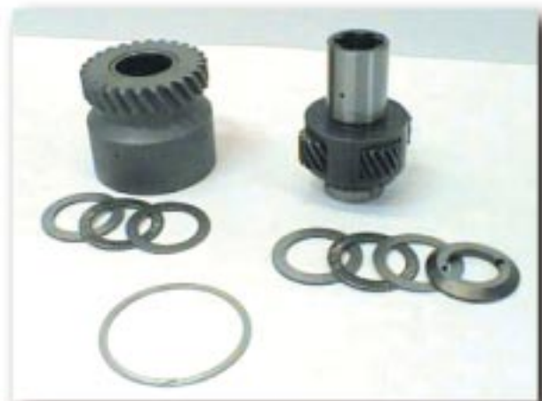
Step P5 Thoroughly clean & inspect all parts for wear. Replace if necessary.
