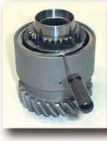
Step P1 Using a small flathead screwdriver, remove the snap ring from the gear housing.
